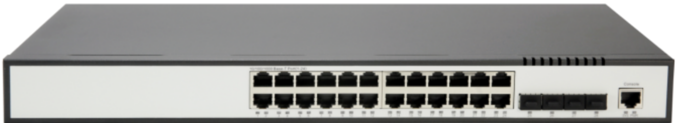
S2624-4X: 24*10/100/1000M Base-T, 4*1000M Base-X SFP/10GE SFP+, Single power supply
